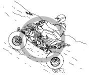
Always check the terrain carefully before you start up any hill. Never climb hills with excessively slippery or loose surfaces. Shift your weight forward.
